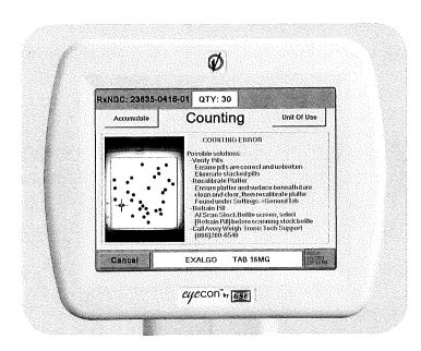
**Counting Errors -** If Eyecon detects objects on the tray that are sufficiently different in size or shape than the pills being counted, a counting error screen is shown. A pill tray photo displays the object(s) in question identified by a red plus sign.
